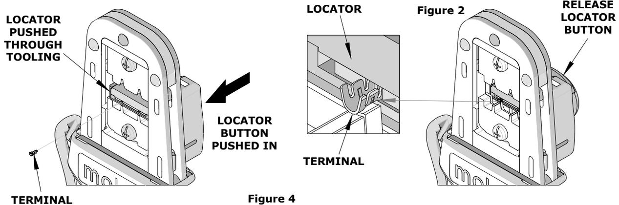
4. Release the locator button, allowing the locator to return to the crimping position.
