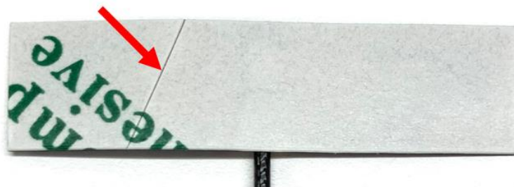
1. Find cut line on flex back side
