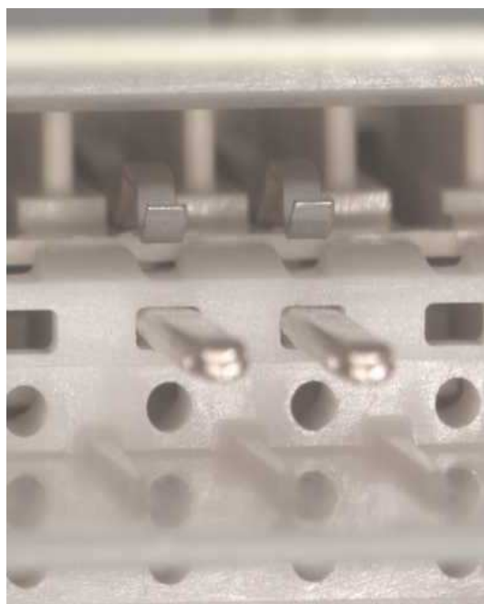
Proper Alignment of Shorting Bar Orientation Feature Un-damaged
