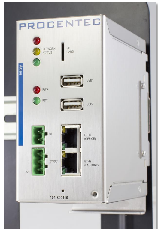
Figure 1 – Atlas mounted on a 35mm DIN
