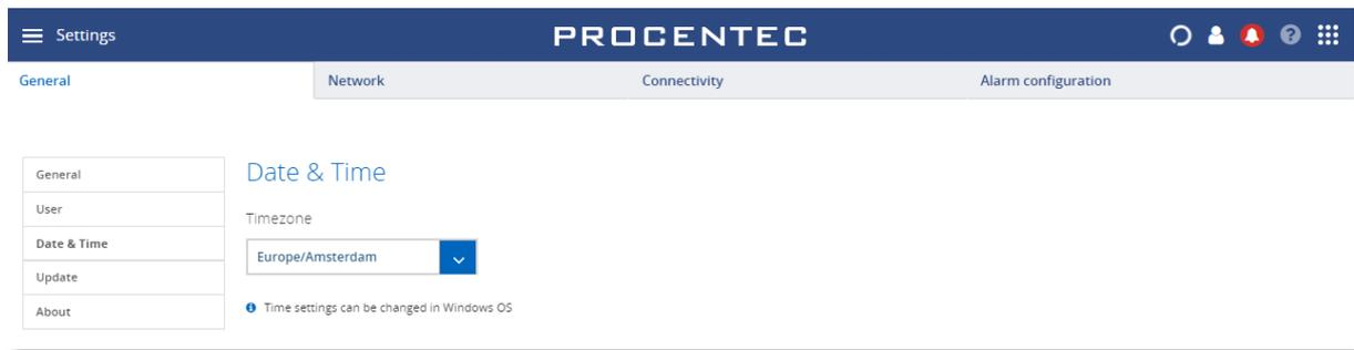
Atlas only: When choosing automatic time, Osiris will try to connect to one of the given NTP servers which require internet connectivity. In case you have a local NTP server(s) then you can remove and replace these defaults servers.
