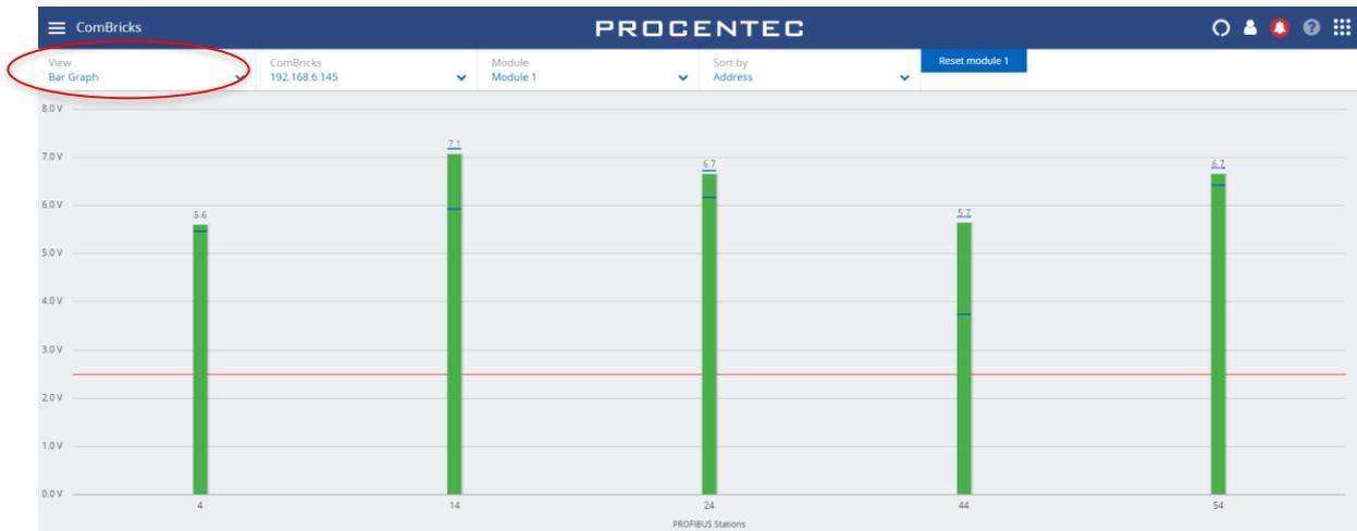
The 'Reset module x' button can be used to clear all Bar Graph data from that module. Resetting the Bar Graph in Osiris will also reset it in the ComBricks.
