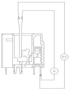
System resistance equals millivolt drop (mV) divided by test current (A) (Conductor resistance will be deducted from measurement).
