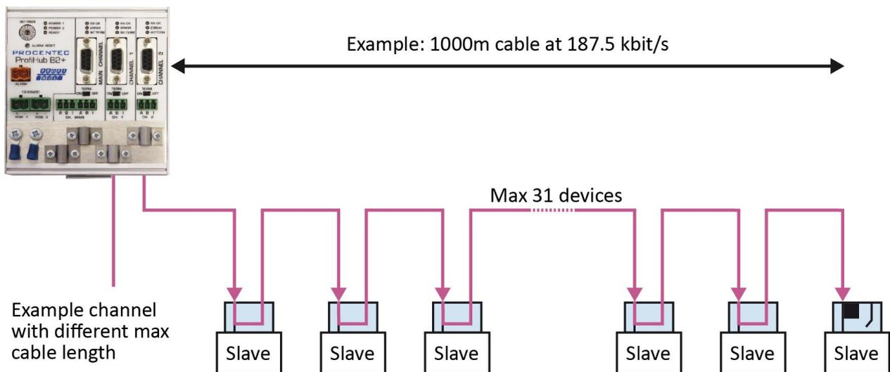
Fig. 6 - Cable lengths for PROFIBUS DP
