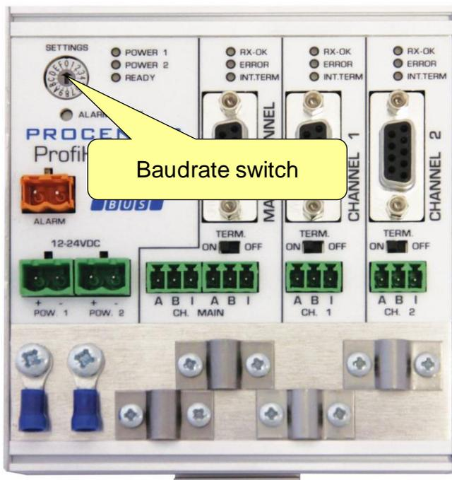
Fig. 16 - Baudrate speed switch
