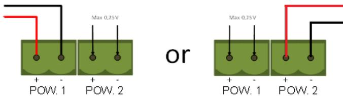
Fig. 11 – Maximum voltage on unconnected Power Connector
