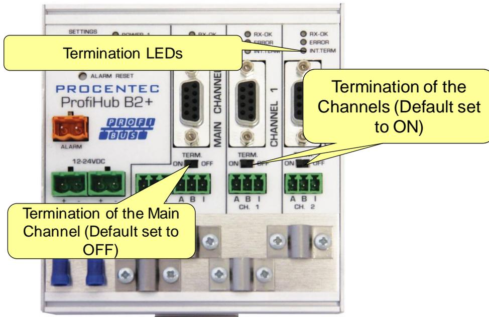
Fig. 15 - Termination Switches
