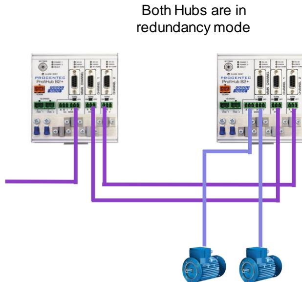
Fig. 17 - Redundant path between two ProfiHubs
