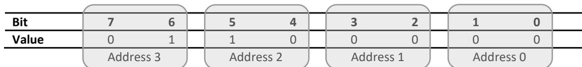
This module also has 2 Output bytes. The first Output byte is used to select the Livelist of a specific Channel. This selection can be read-back in the Input byte described above.
