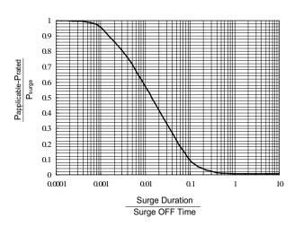
Pulse load rating in accordance with IEC 60115-1, 4.27  $1.2\mu$ s/50 $\mu$ s; 5 pulses at 12s interval for  $\pm$ 0.5% resistance change
