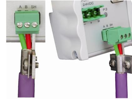
Fig. 4 Using the Ground Clip
