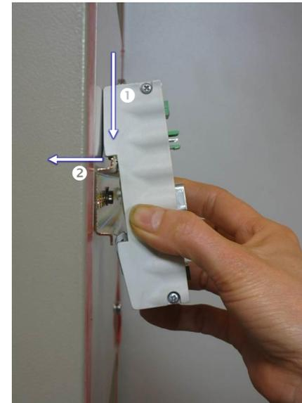
Fig. 1 Mounting; pull-down and push
